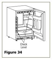
If the ice maker is not level, adjust the feet on the corners of the unit as necessary (see Figure 35).
